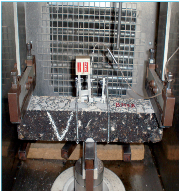
Photo 2. Three-point bending flexural test
