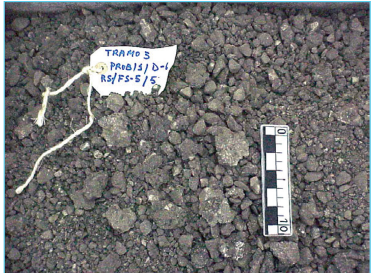
Photo 2. Example of milled material in Spain, obtained in one of the tests of the SCORE project
