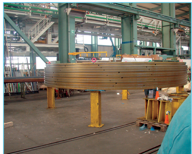
Photo 6. Rotary coupling, incorporating water, foam or polymer piping
